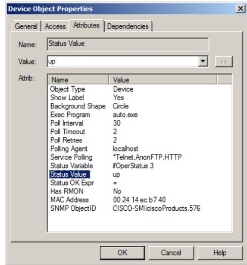
**Note:** For variables that have a textual instance part, you can use the form *statusVar."text instance"* rather than full SNMP dot notation.
