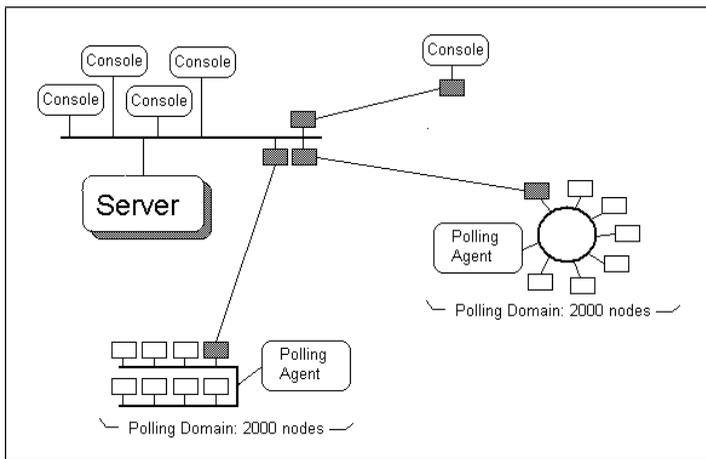
SNMPC Enterprise uses the popular SNMP management protocol to poll and configure devices, workstations and servers over IP networks. Along with all the features expected in any SNMP management station, SNMPC Enterprise also includes the following advanced features:
