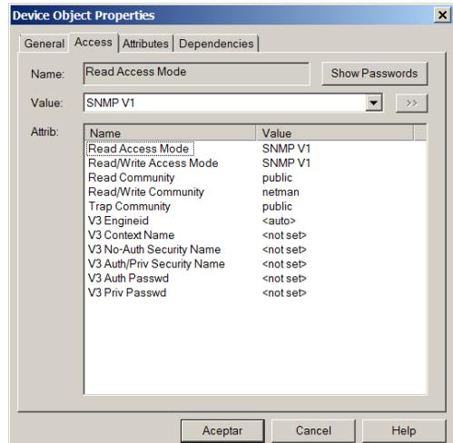
The following table describes the access parameters available in the **Object Properties Access** tab for **Device**, **Link**, and **Network** objects. Access parameters are not valid for Subnet and Goto object types.
