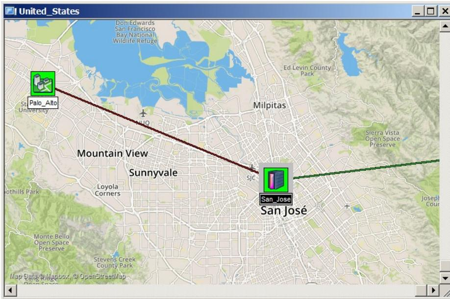
Use the **Latitude, Longitude** attribute of the **Object Properties** dialog to move any device object within a Geo Subnet map view to a specific GPS or street address location.
