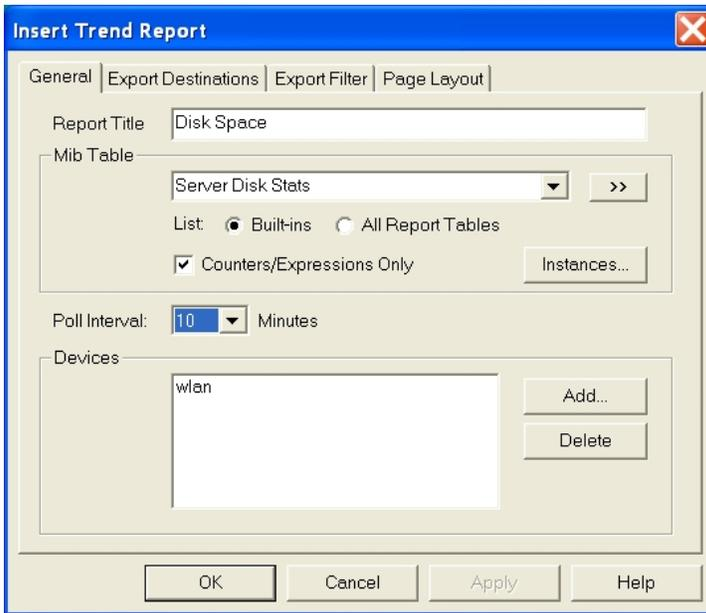
4) To configure a threshold on the data being recorded select the *Instances...* button.
